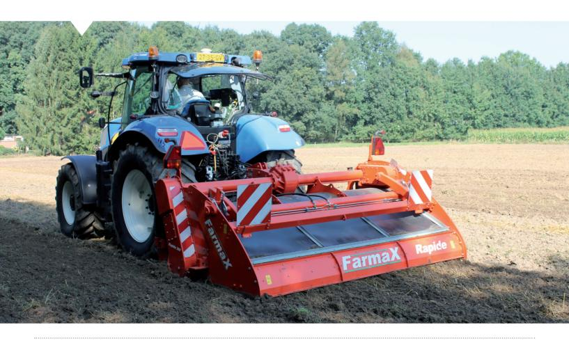
The Farmax Rapide tills heavy sand, clay and even stony soils quickly and without problems. The Rapide is a very heavyweight design and has PE plating to prevent clogging of the machinery.
