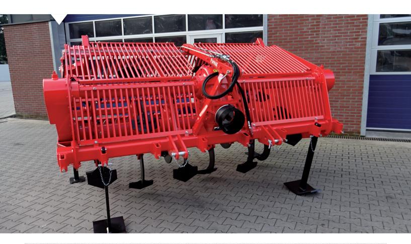
Farmax deep spaders are designed for extra-deep soil working and for breaking and mixing hard layers.
