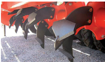
The spader blades are attached with shearing bolts
