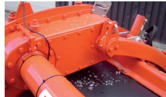
Intermediate drive for narrow transport width
