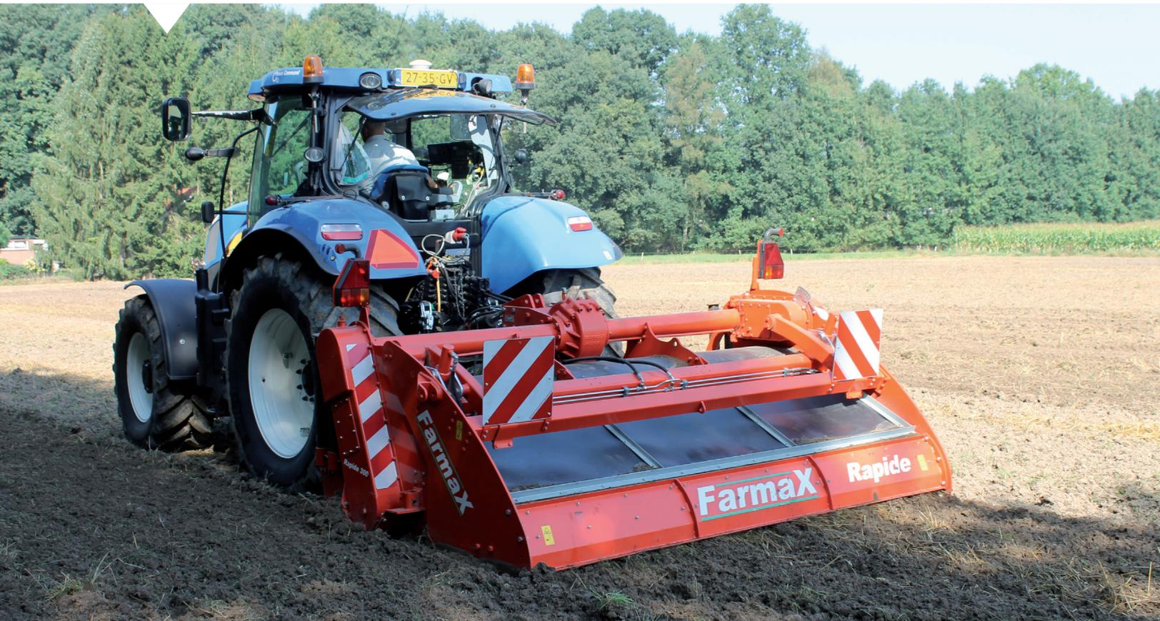
**The Farmax Rapide tills heavy sand, clay and even stony soils quickly and without problems. The Rapide is a very heavyweight design and has PE plating to prevent clogging of the machinery.**
