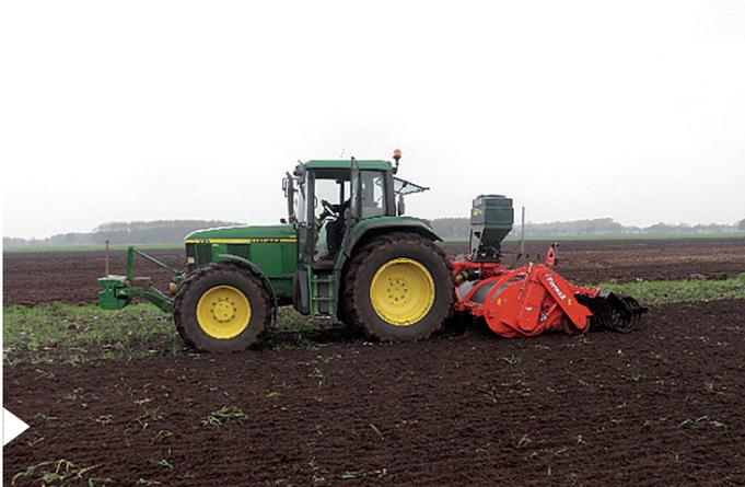
The PE covering prevents the machine getting blocked up. With this spader, structural damage, such as a plough pan or compaction of the subsoil, is a thing of the past. Altogether, this results in a 10-20% increase in crop yield.
