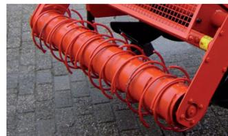
Rotary harrow ensures an optimum bed for sowing
