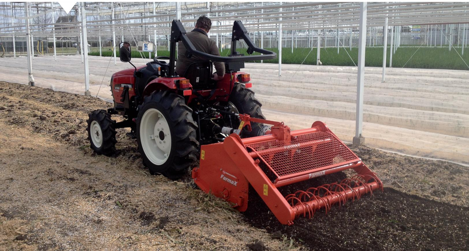
The Farmax ERP is a spader for light tractors. The great manoeuvrability and low integral weight of the ERP make it highly suitable for use in greenhouse horticulture, flower cultivation and tilling small plots.
